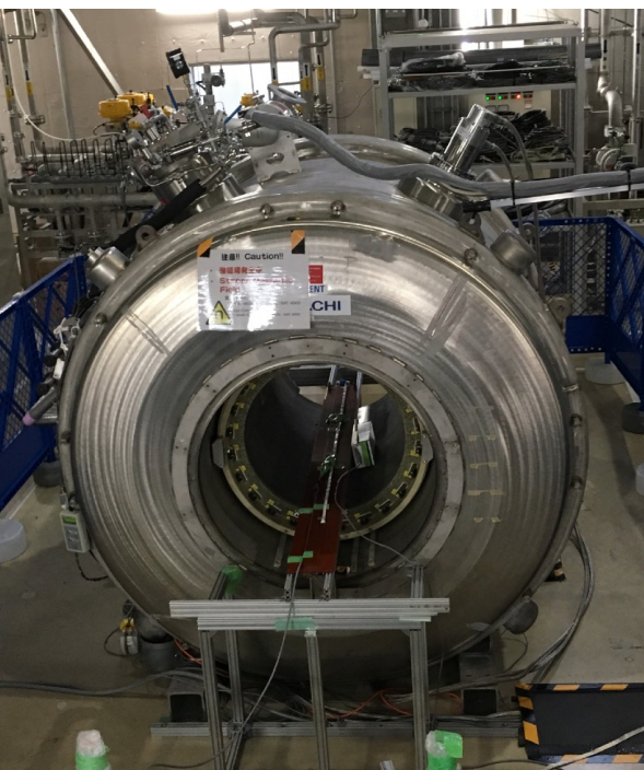
Superconducting magnet: 1.2 T Axial length: 2 m, Bore diameter: 925 mm.
