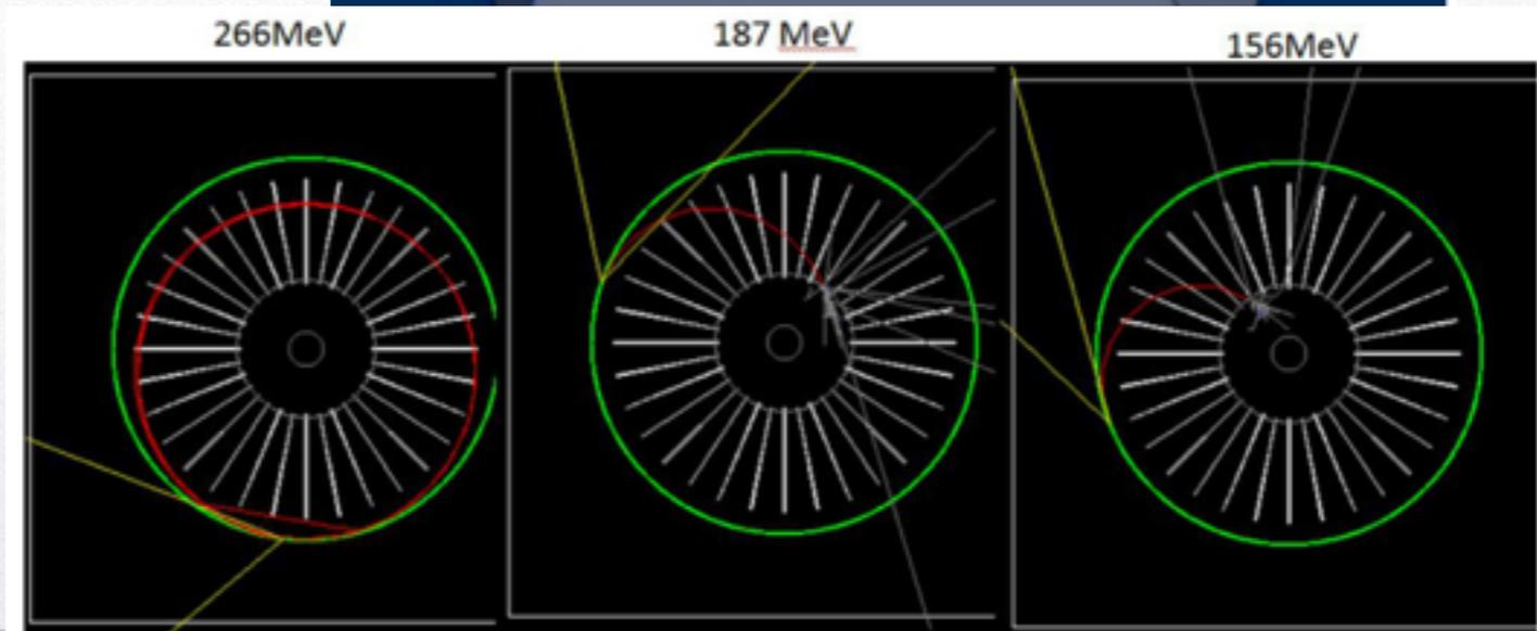
**Figure 6:** Example positron trajectories in the detector system at three different energies of positrons. The green circle is the muon beam orbit. The red trajectory is the trace of the positron track. The white tracks are photons.
