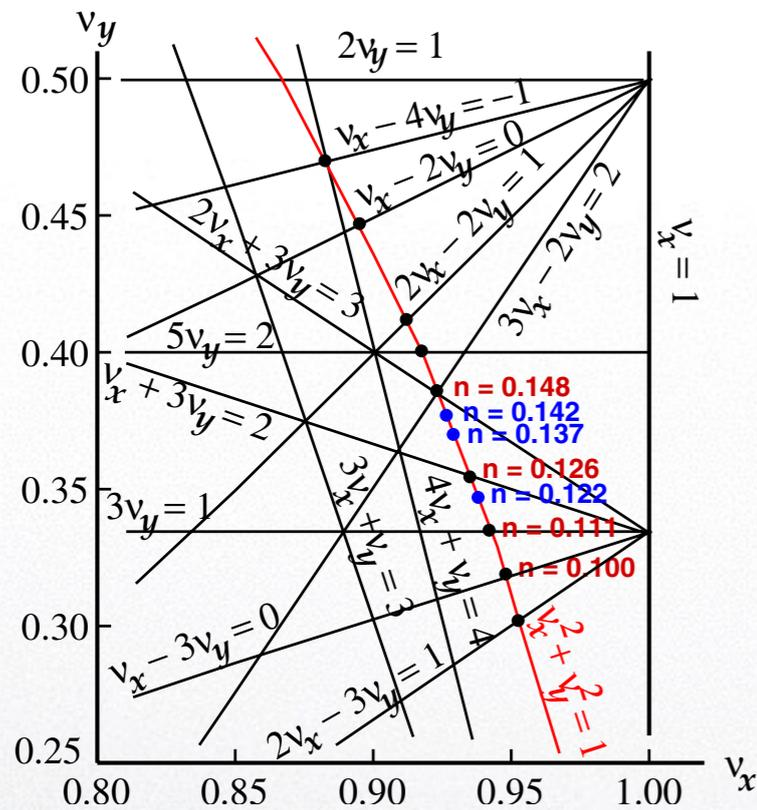
FIG. 18 (color online). The tune plane showing resonance lines. Three of the  $n$  values used to run the experiment, 0.122, 0.137, 0.142, are indicated on the arc of the circle defined as  $v_x^2 + v_y^2 = 1$ . They do not intersect any of the resonance lines, contrary to nearby tunes, which are also shown on the arc.
