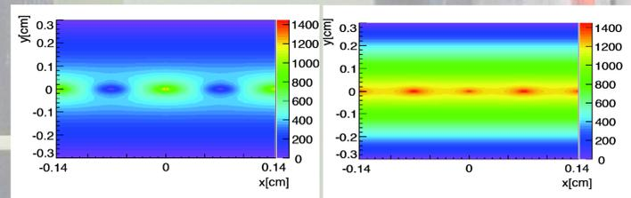
Potential gradient of the electric field when 1450 V is applied across potential wires (right) is smaller than that when 0 V is applied (left).
