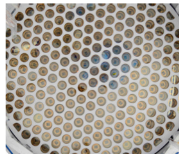
PMT array (494 PMTs in total, in 2 arrays)
