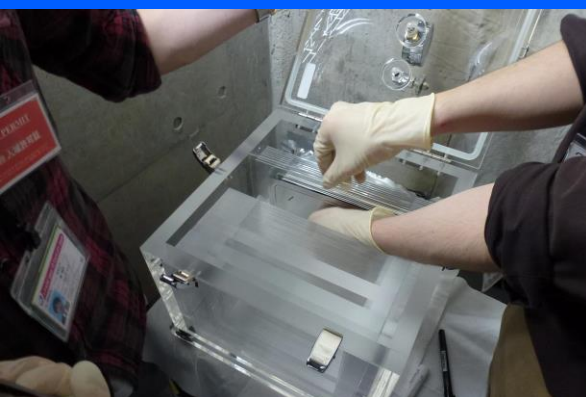
Sandwich structure of Emulsion films and Frame type spacers
