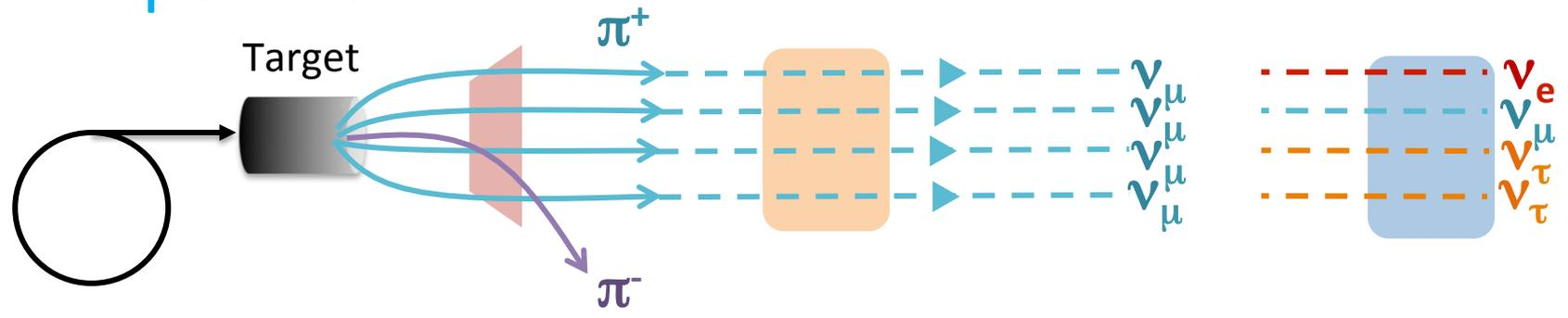
Proton Accelerator      Magnetic Horns      Near Detector      Far Detector
