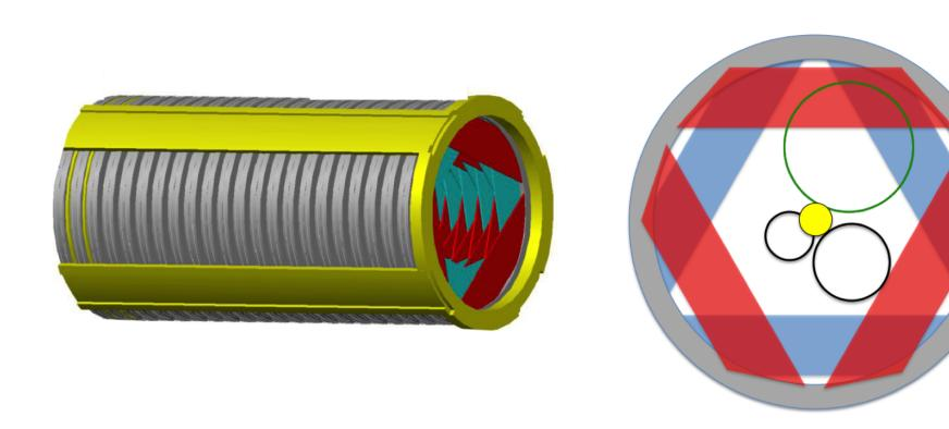
The tracker consists of a low mass array of 21600 straw drift tubes in 18 tracking stations to measure the trajectory of charged particles in a uniform magnetic field of 1T.
