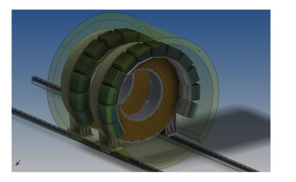
The calorimeter consists of two disks, each composed of ~900 BaF<sub>2</sub> scintillating crystals each read out by two avalanche photodiodes. The calorimeter contributes to the PID and trigger, and can independently confirm measurements by the tracker.
