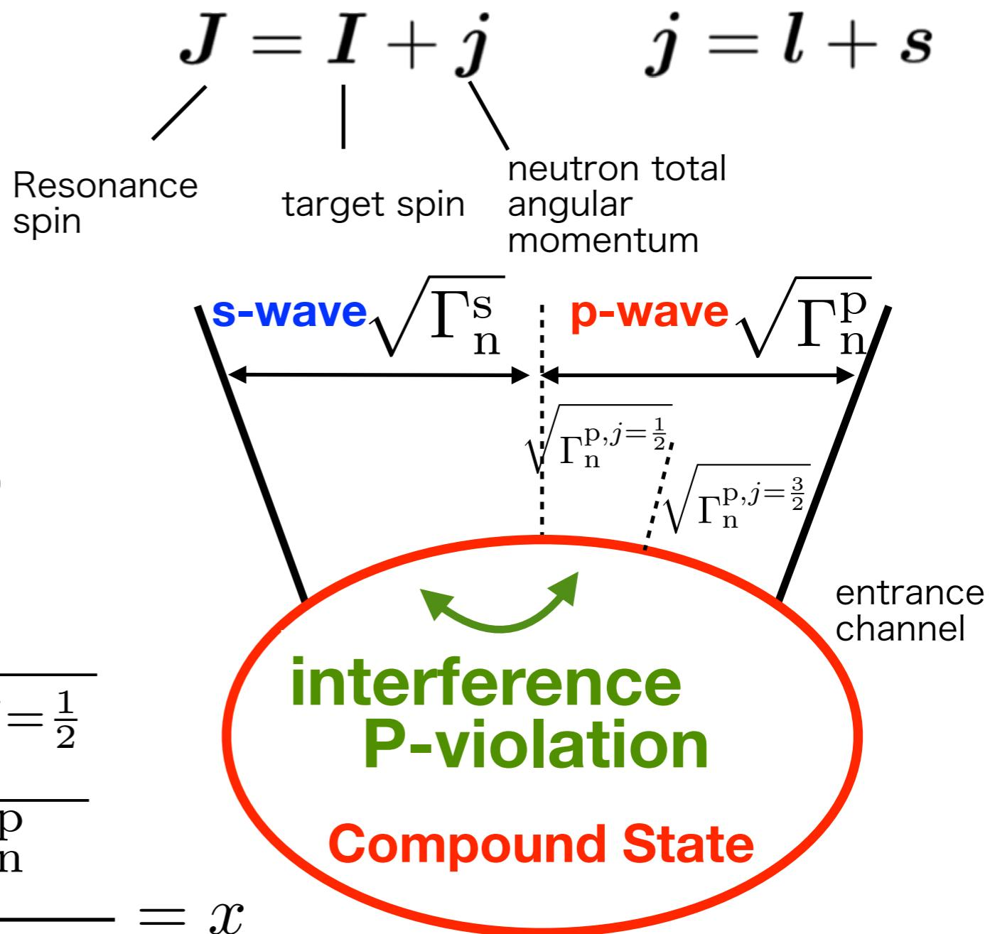
$$A_L = -\frac{2W}{E_p - E_s} \sqrt{\frac{\Gamma_n^s}{\Gamma_n^p}} \sqrt{\frac{\Gamma_n^{p,j=\frac{1}{2}}}{\Gamma_n^p}} = x$$
