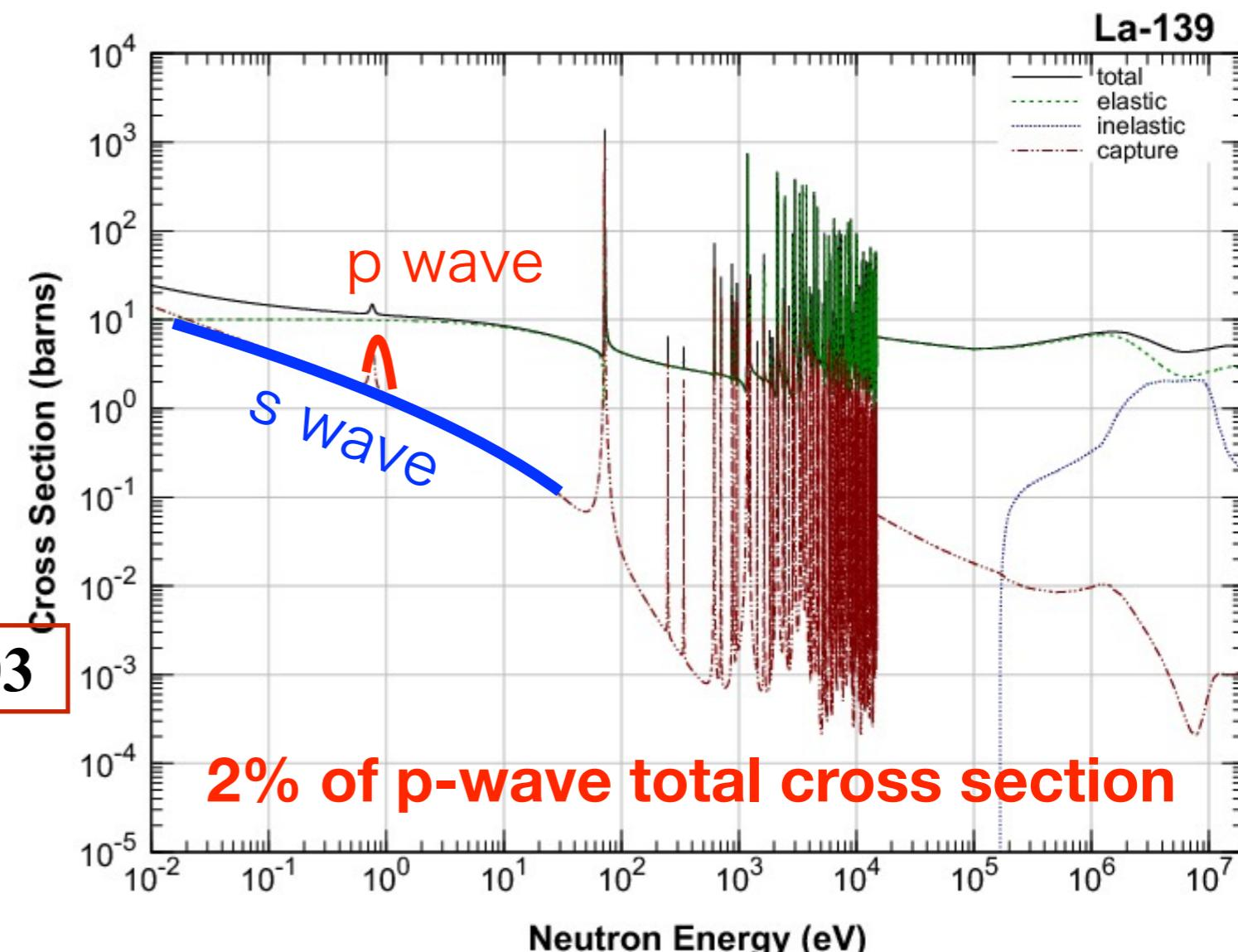
P-violation is enhanced in the interference between s-wave and p-wave of compound nuclei.
