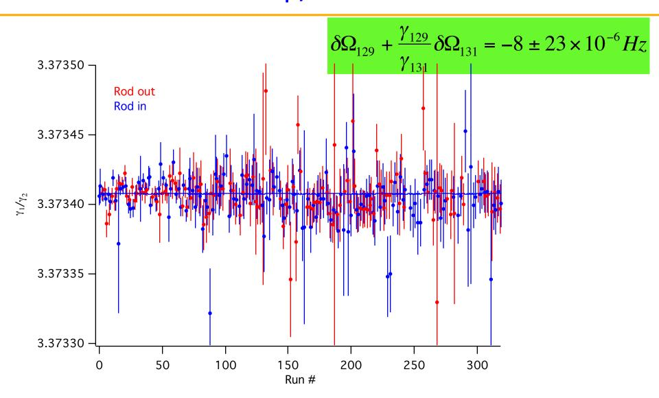
Frequency shift zero at 2E-5 Hz level in ~3-day experiment on their "test" apparatus Apparatus improvements can achieve ~1E-9 Hz precision
