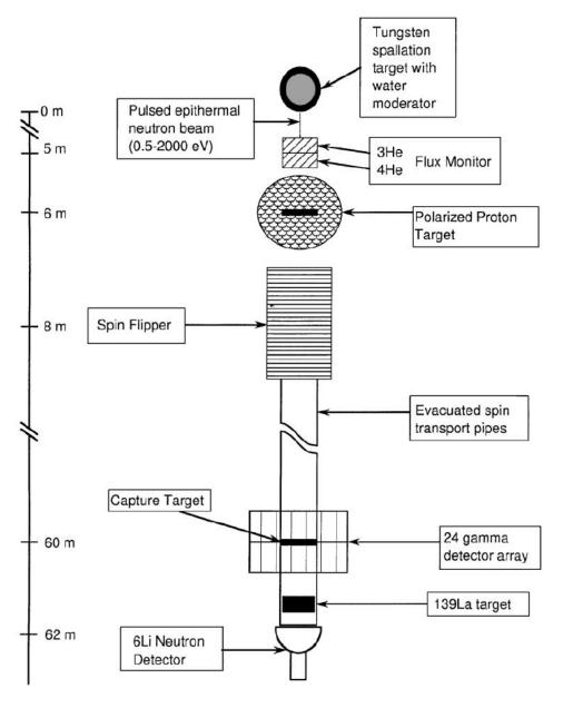
Apparatus for PV at a spallation neutron source
