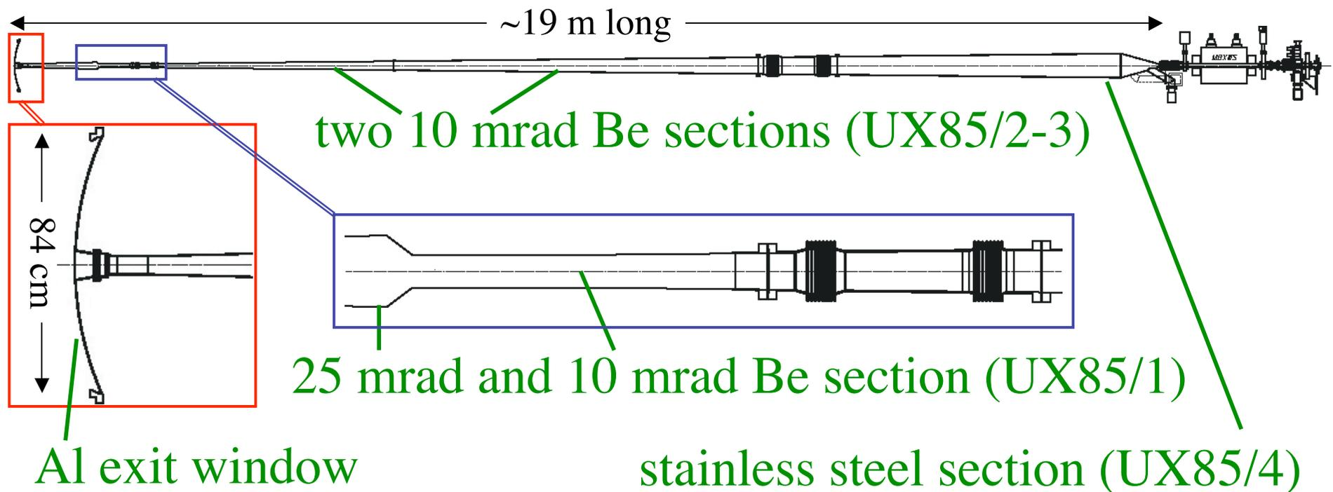
All the beam pipe sections delivered to CERN.
