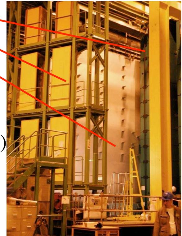
Projective readout based on MWPC's except 3-GEM at M1R1 (high occupancy)
