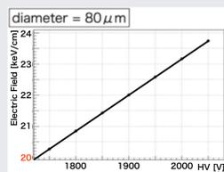
Fig5. Surface E field of field wire
