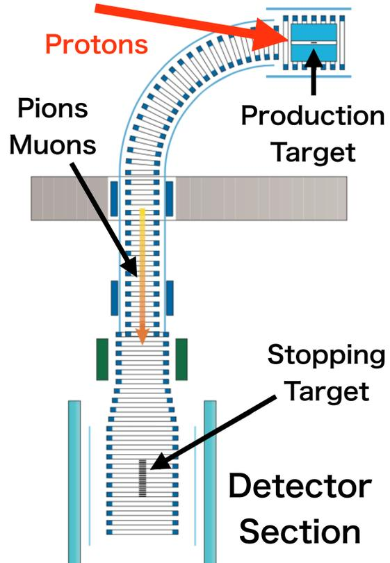
Fig1. Schematic of COMET Phase-I
