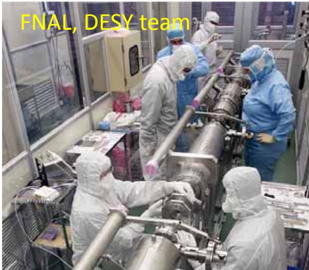
cavity connection in clean room for module installation
