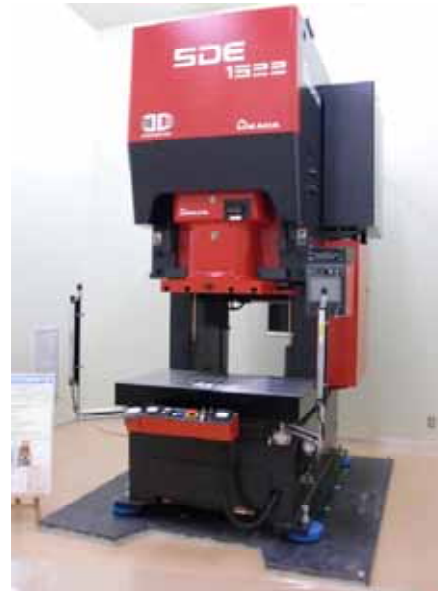
AMADA digital-survo-press SDE1522 150t, 50stroke/min, 225mmstroke
