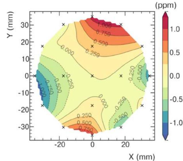
At  $\sim 8000$  azimuthal locations, obtain a field contour plot from the 17 probes
