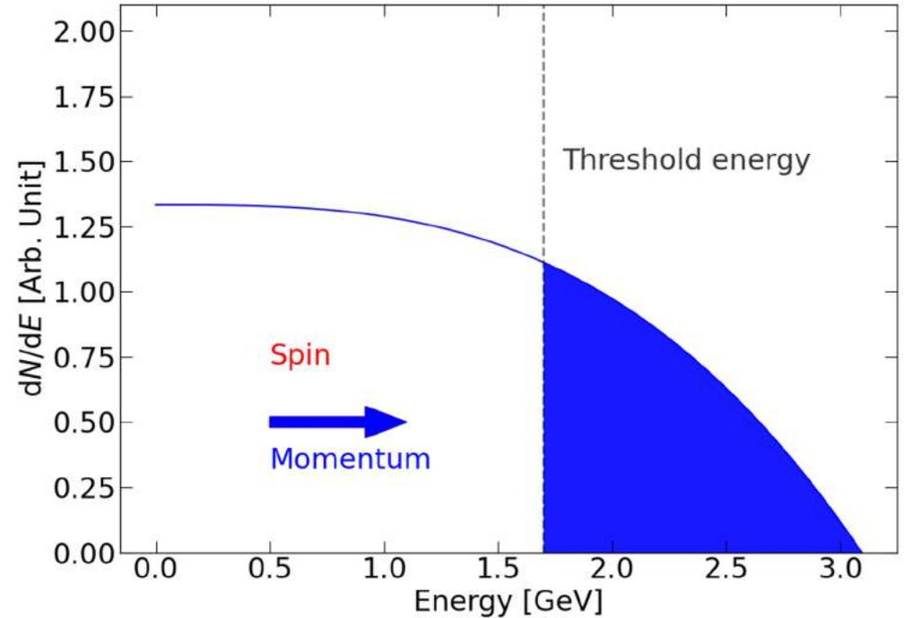
The number of high momentum positrons above a fixed energy threshold oscillates at precession frequency
