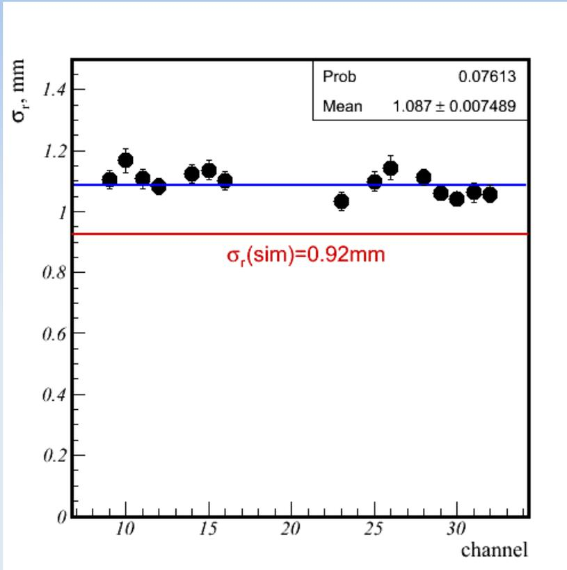
Difference between  $\sigma_r$  and  $\sigma_r(\text{sim})$  comes mainly from track resolution ( $\sim 0.5 \text{ mm}$ )
