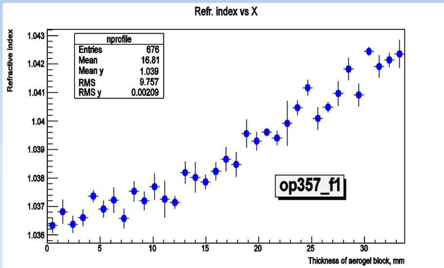
$n(x)$  dependance was measured using digital x-ray detector
