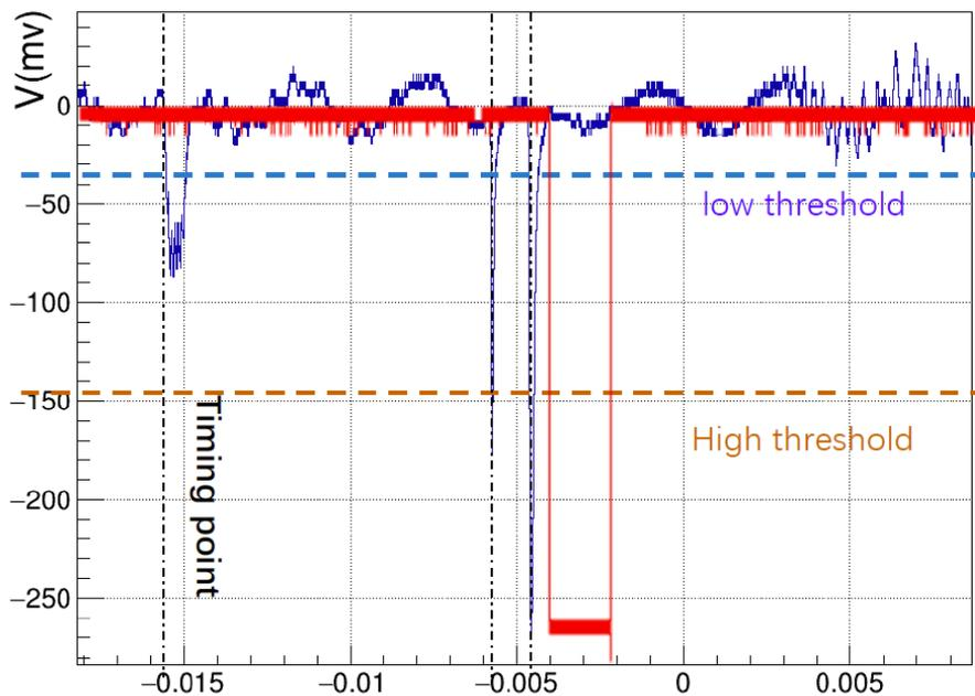
— Fast loss monitor waveform
