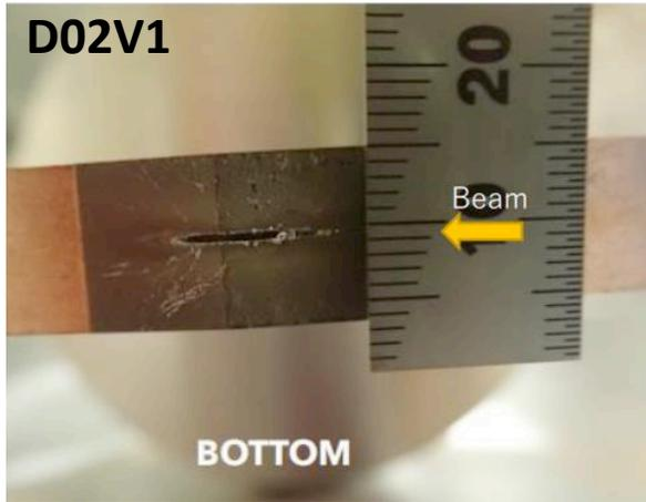
Severe damage on D02V1 collimator heads after QCS quench with high beam current.
