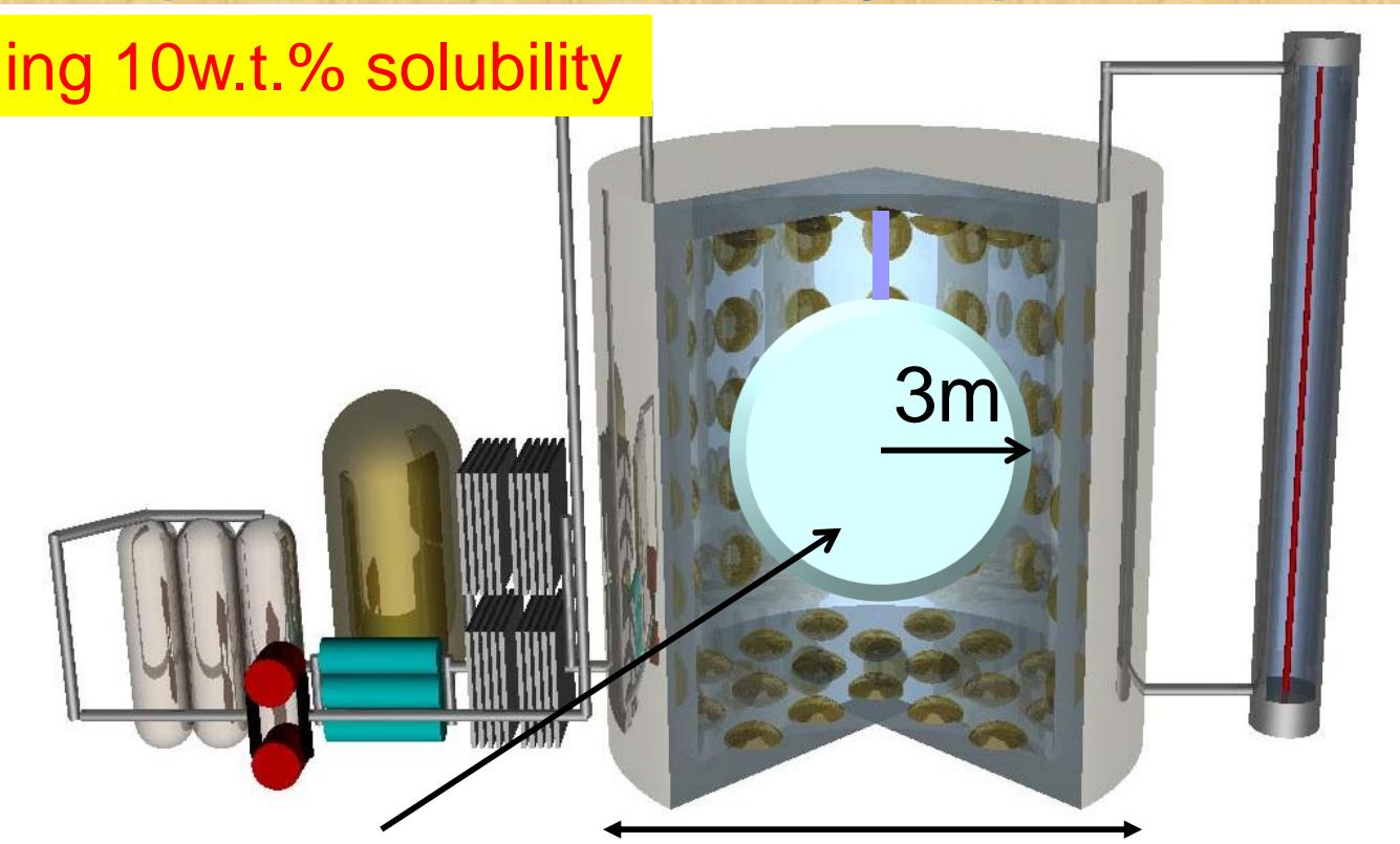
Zirconium loaded 100ton LS
