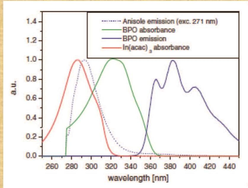
Same overlap between the emission and the absorption could be occurred even if different metal (Zr) was used.
