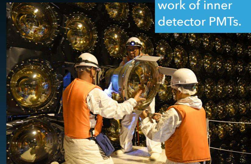
Replacement work of inner detector PMTs.
