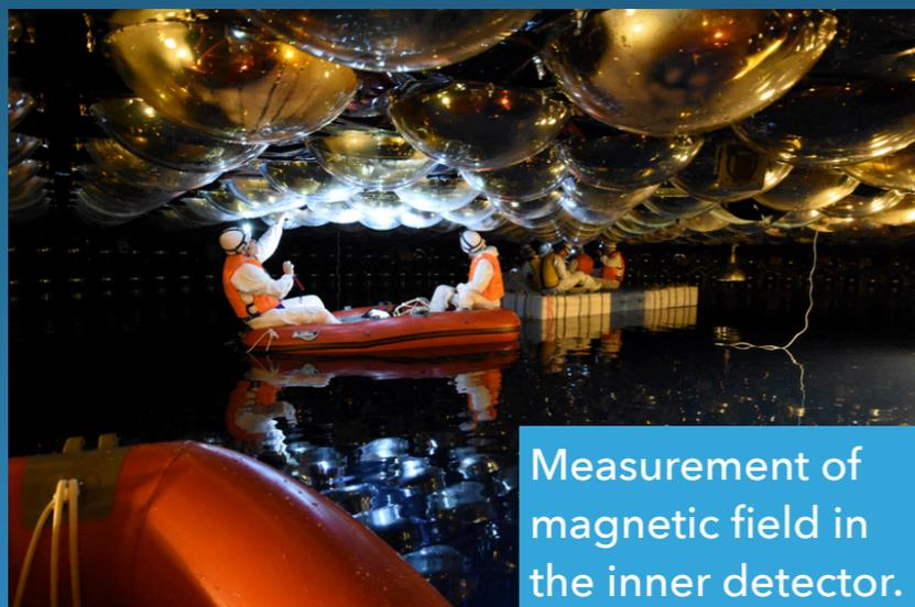
Measurement of magnetic field in the inner detector.
