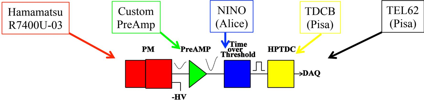
The contribution of the FE electronics and of the DAQ to the time resolution is lower than 50 ps
