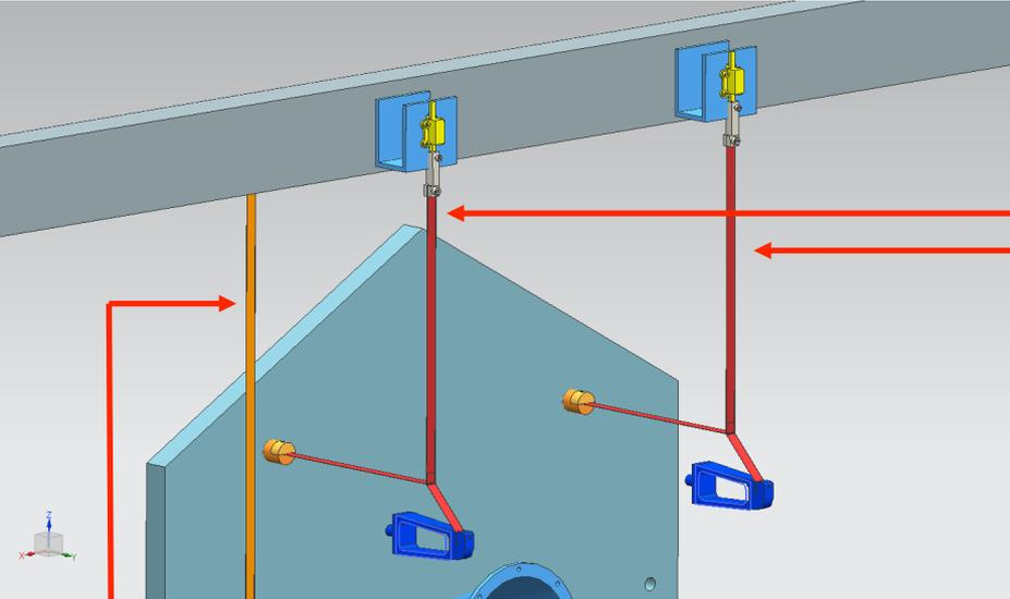
The orientation of the mirrors is remotely adjustable using piezo-motors
