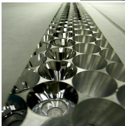
Detail of Winston Cones with and without Mylar foils
