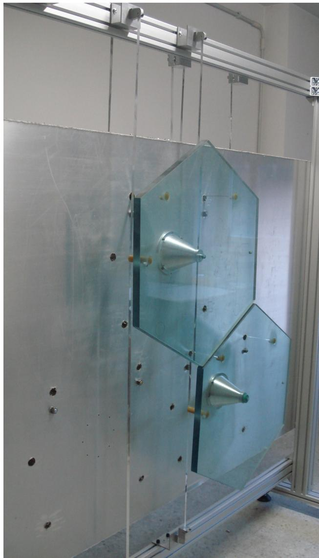
A prototype of the support with 3 mirrors is under construction
