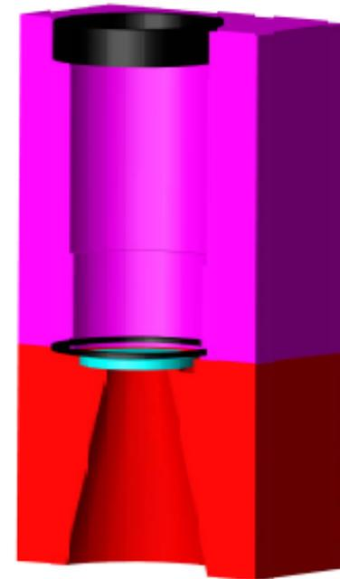
Neon-air separation disk (Quartz window side)
