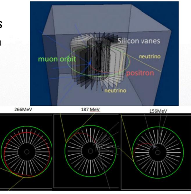
Figure 6: Example positron trajectories in the detector system at three different energies of positrons. The green circle is the muon beam orbit. The red trajectory is the trace of the positron track. The white tracks are photons.
