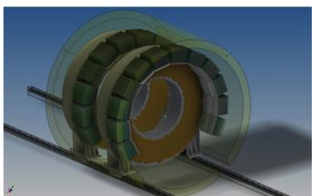
The calorimeter consists of two disks, each composed of ~900 BaF<sub>2</sub> scintillating crystals each read out by two avalanche photodiodes. The calorimeter contributes to the PID and trigger, and can independently confirm measurements by the tracker.
