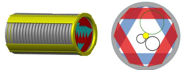
The tracker consists of a low mass array of 21600 straw drift tubes in 18 tracking stations to measure the trajectory of charged particles in a uniform magnetic field of 1T.
