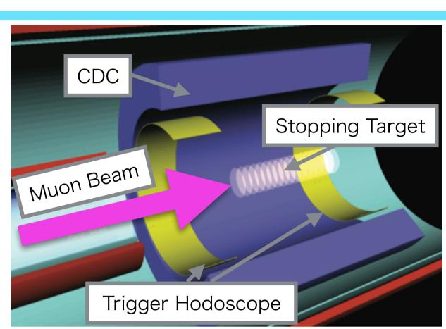
Fig3. Schematic of detector section
