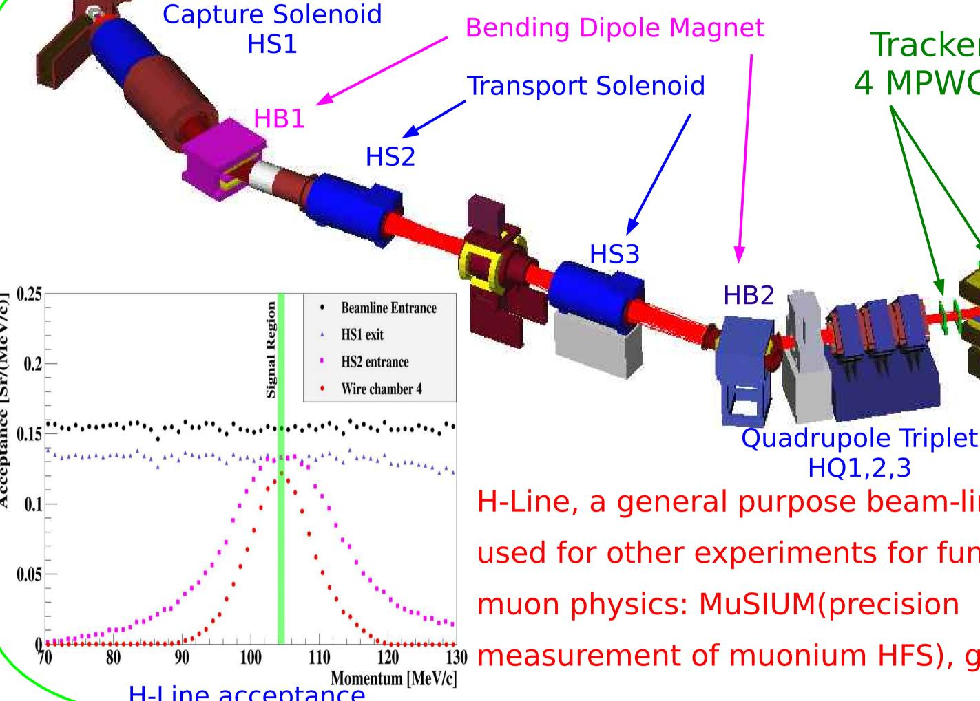
magnet HQ1,2,3 H-Line, a general purpose beam-line, can be used for other experiments for fundamental
